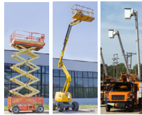
A scissor lift (left), a cherry picker (middle), and a bucket truck (right).
