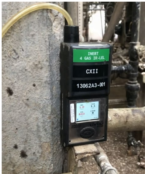
Figure 2. O 2 concentration monitoring in the FCC main column overhead stream during non-normal operation
