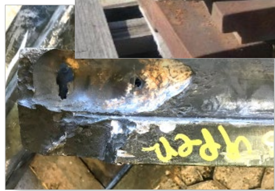
Damage consistent with continuous use of guide purge
