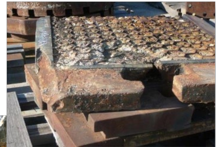
Damage consistent with continuous use of guide purge
