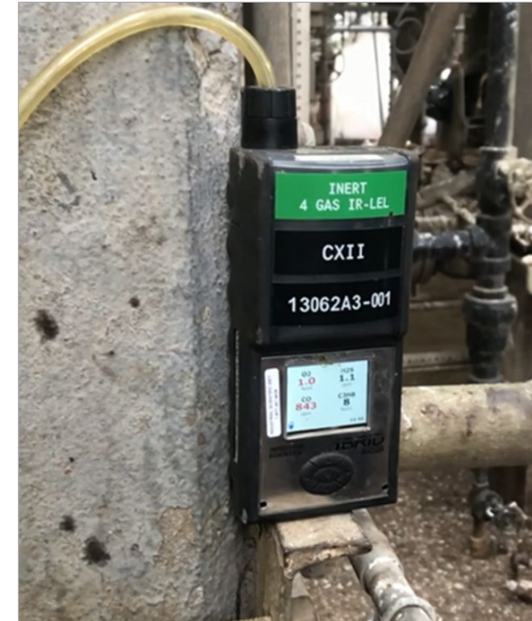
O 2 monitoring in the FCC main column overhead stream during non-normal operation.
