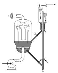
Cause – Feed not diverted from Riser or Torch Oil injected below ignition temp.
