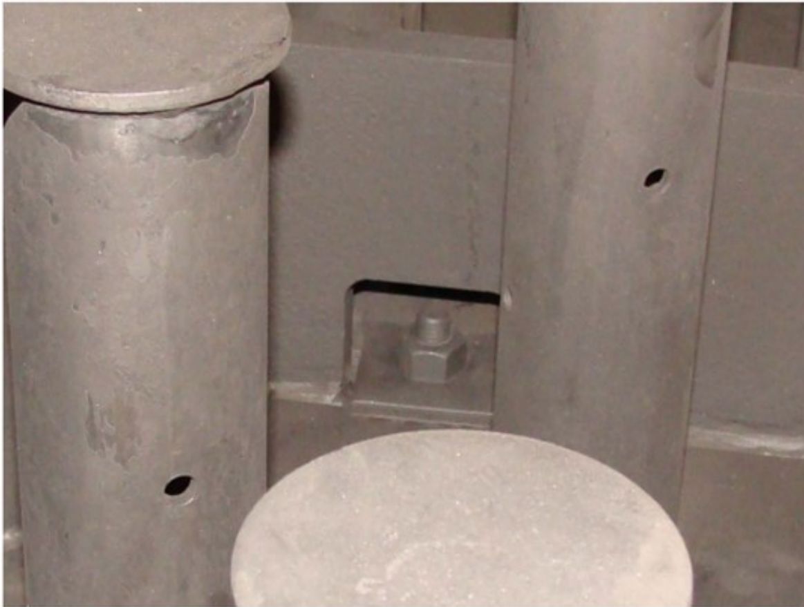
Top Tray Liquid Distributor – Close up after CO 2 Blasting
