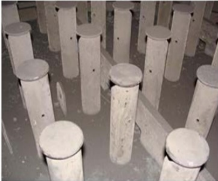
Top Tray Liquid Distributor – Overview prior to cleaning
