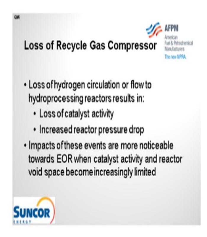
At Suncor, we have found several effective methods for minimizing the impact of loss on our hydrogen recycle gas compressor. First, we stop the flow of feed and depressure the reaction section. This action clears as much of the oil off of the hot catalyst as possible to avoid coking reactions that occur in low hydrogen partial pressure environments.
