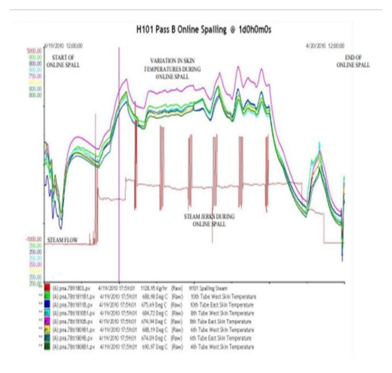
We use a combination of BFW and steam as spalling media, with BFW injection at convection inlet to cool convection section properly. Combined flue gas continues to be hot from other passes, which are operating as usual and BFW helps cooling the convection section of the pass being spalled. Steam is injected at the cross- over.
