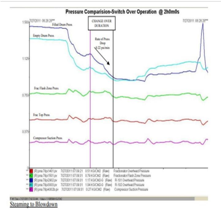
Once steaming towards fractionator is over, the steam and residual vapour from the drum overhead is routed to the blowdown system and steaming is ramped up to 16-18 t/hr (28 ft Coke Drum) and continued for 1.0 hr. If this switch to blowdown is performed too fast, it might again cause a sudden pressure drop in the drum which might uplift the foam bed. In some instances, foam and other material have been sucked in the drum vapour line and caused severe fouling and plugging.
