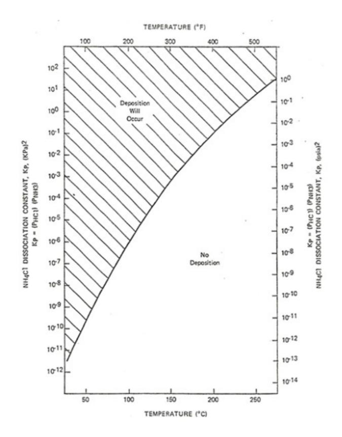
It is critical when using intermittent water wash to remove the salt deposits completely as introducing water in the presence of these salts can result in excessive corrosion leading to potential loss of
