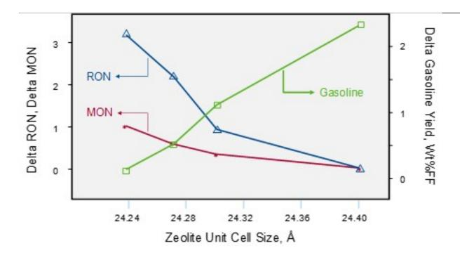
The impact that the FCC catalyst can have on gasoline octane is demonstrated through a recent Grace publication.6 The refinery switched from an alternate supplier to a Grace catalyst with an optimized UCS, which led to an increase in the FCC gasoline MON by 0.5 numbers that enabled the refinery to produce 5% more premium-grade gasoline.
