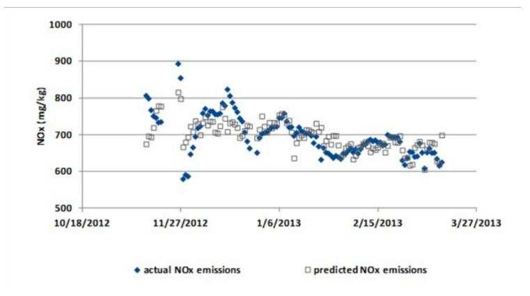
Figure 5 shows how the NOx emissions decreased when switching from the platinum-based promoter to CP® P.
