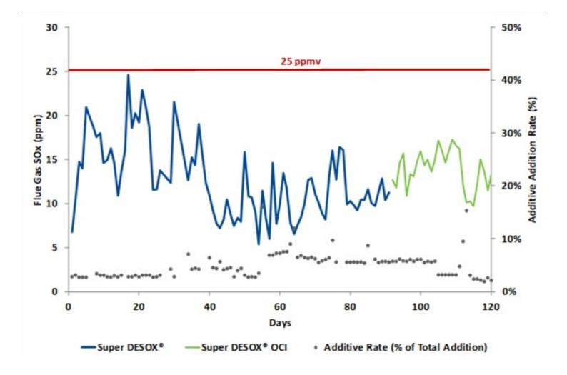
Figure 1: Both Super DESOX® and Super DESOX® OCI additives-controlled SOx to <25 ppmv
