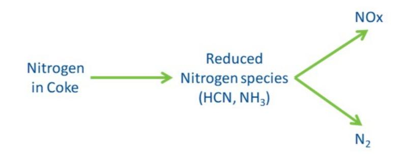
Grace offers two types of catalytic additive technologies for reducing NOx levels in the FCC unit: low NOx combustion promoters and standalone catalytic NOx reduction additives.
