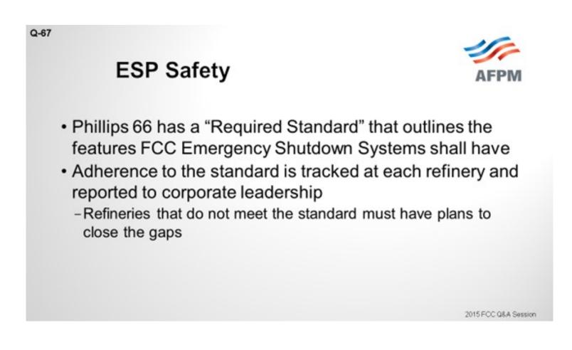
One of the features required by this standard is that the ESP shall shut down if the main FCC safety system engages or trips, regardless of the cause. There are several other features. If the inlet CO (carbon monoxide) level exceeds the prescribed limit in the standard, which says that it can be no
