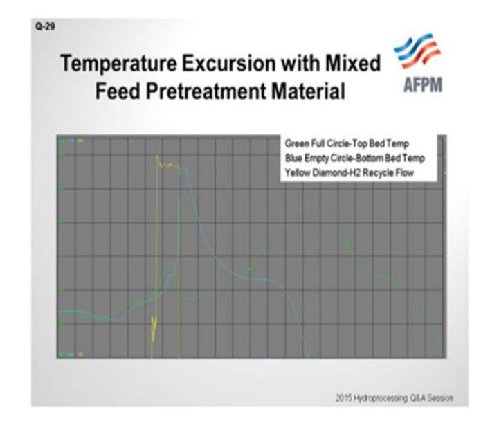
In addition, the catalyst was very dry after prolonged nitrogen circulation, and it is believed that the water generated by the reverse reaction was absorbed by the catalyst causing it to heat up, which initiated a reduction reaction that lead to the temperature excursion. Stopping the hydrogen flow discontinued all of this, and we are able to get back down to a safe level. According to the supplier, this was the first observation of such an issue with this material.
