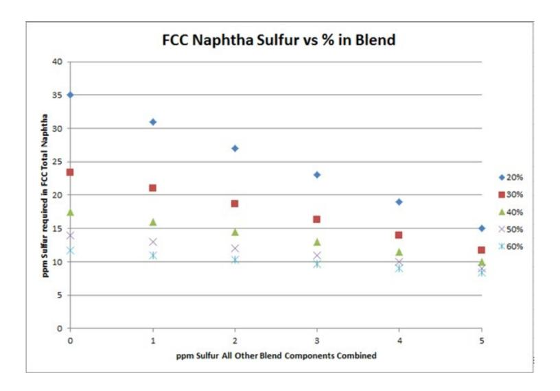
The degree of hydrotreatment of FCC naphtha is dependent upon several factors, including the sulfur content of the feed to be treated, relative amount of FCC naphtha in the pool, and combined sulfur of all other blend components.
