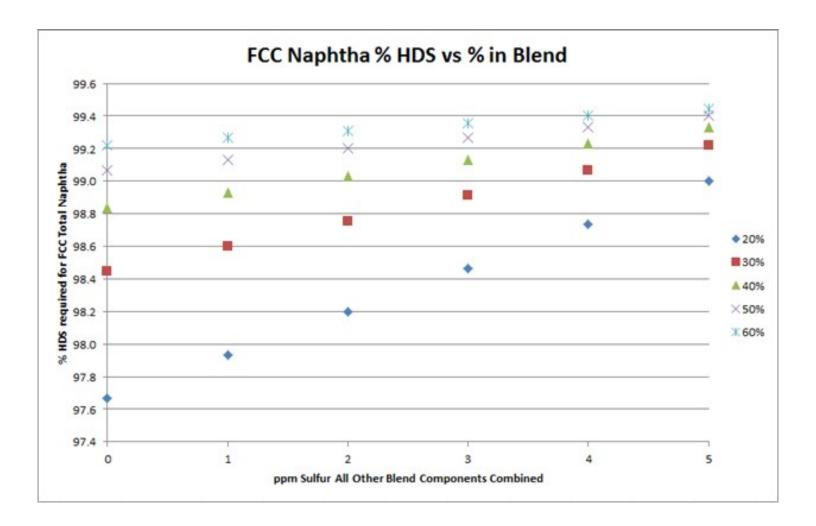
The plot above shows that the lower the sulfur of the blend components other than FCC naphtha, the lower the extent of hydrodesulfurization required for the FCC naphtha.
