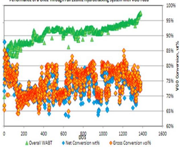
Performance of a Once Through Full Zeolite Hydrocracking System with VGO Feed
