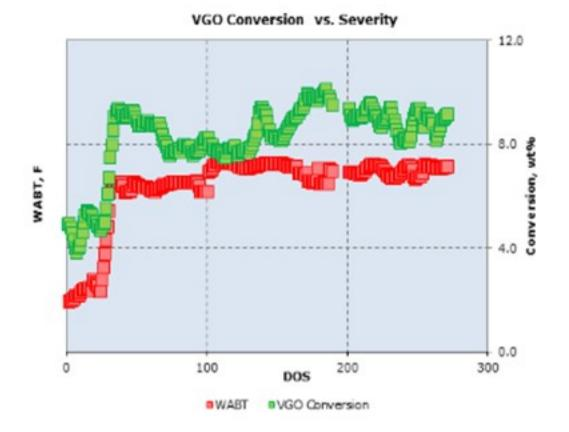
When higher levels of conversion are desired, addition of a catalyst to provide mild hydrocracking is needed. Our customers are operating many units with MHC catalysts in this mode. When higher distillate selectivity is desired, an alumina/ASA catalyst system can be considered. If even higher
