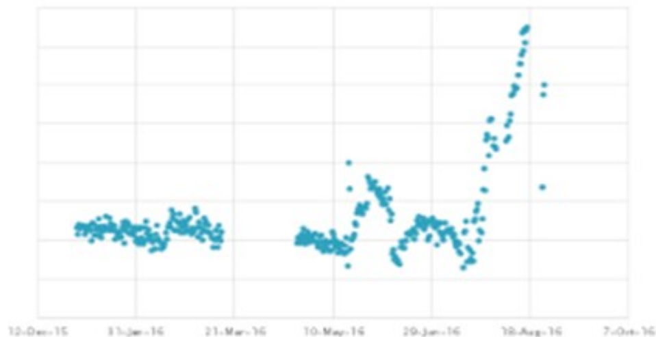
Figure 2. MPC Refinery Bed 3 Inlet Radial Temperature Spread
