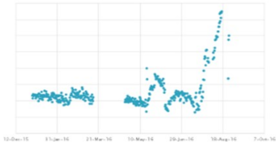
Figure 2. MPC Refinery Bed 3 Inlet Radial Temperature Spread
