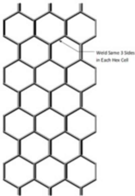
Figure 1: Hex Mesh Welding Diagram in Severe (Coking) Service
