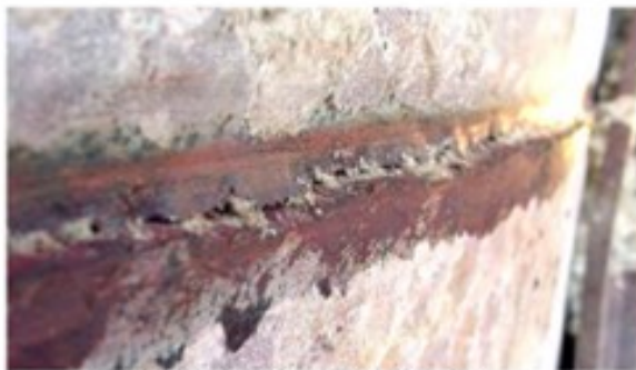
Circumferential weld seam cracking
