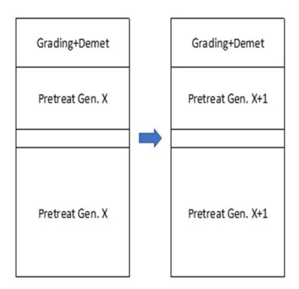
The increased activity of the pretreat system changes shown above enable the replacement of one bed of hydrocracking catalyst in the bottom bed of the hydrocracking reactor with a more middle-distillate cracking catalyst as shown below:
