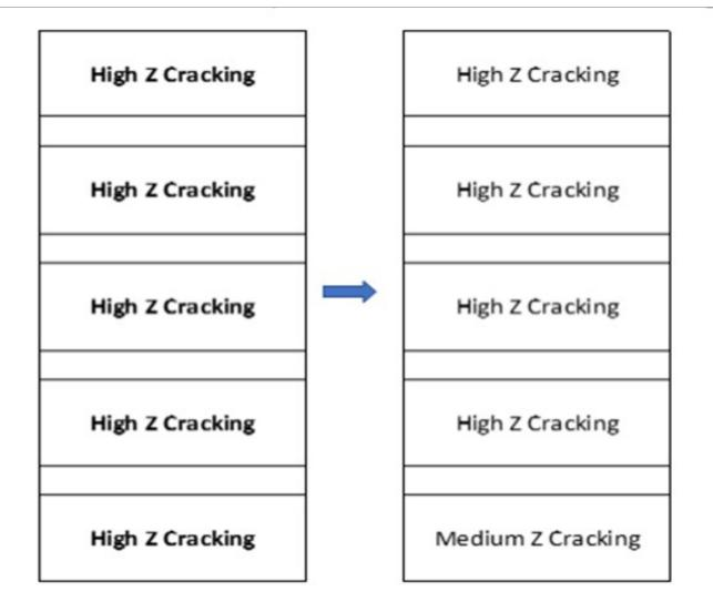
This one bed of more mid-distillate selective catalyst buys a significant improvement in middle distillate yield by virtue of its placement in the highest conversion environment in the reactor. It can be seen from the following comparison that the selectivity advantage of going to a somewhat lower activity, more mid-distillate selective catalyst, in the bottom bed results in a large boost in the marginal increase in middle distillate in this range of 60-70 lv% conversion.
