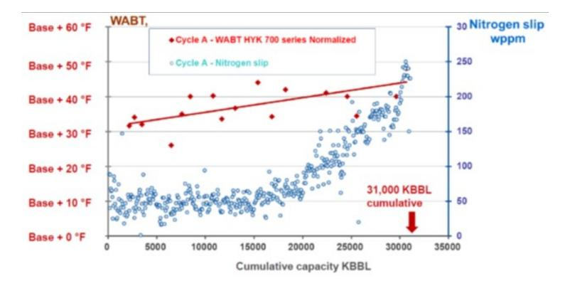
Alternatively, with this increased nitrogen tolerance, the pretreat catalyst volume could potentially be decreased as HDN activity requirement is reduced. Coupling this with current generation higher relative volume activity (RVA) pretreat catalysts, there can be an even more substantial reduction in required pretreat catalyst volume. As discussed previously, this decrease in pretreat catalyst volume can allow for an increased volume of grading, guard, and hydrocracking catalysts.
