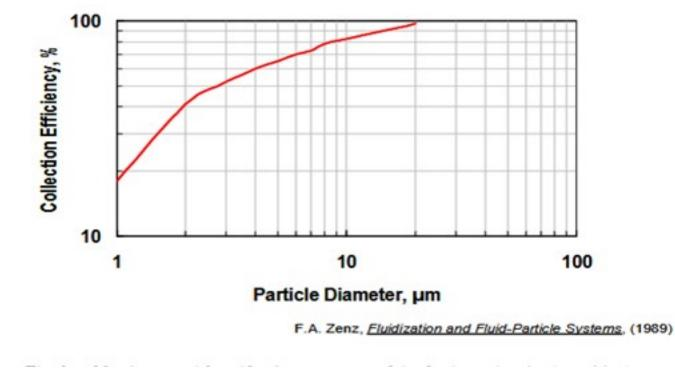
Cyclone Efficiency vs. Particle Diameter
