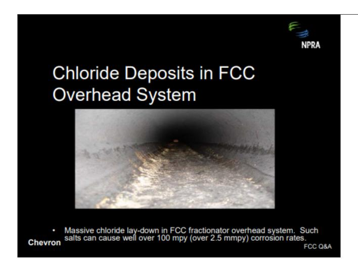
The next picture was taken at a point where we actually opened up the line. It shows the salt deposits at the bottom. The interesting thing here is the hydrocarbons are actually protecting the salt layer so that the corrosion was not as high as you might have expected because the hydrocarbon tend to keep the water out of the salt deposits.
