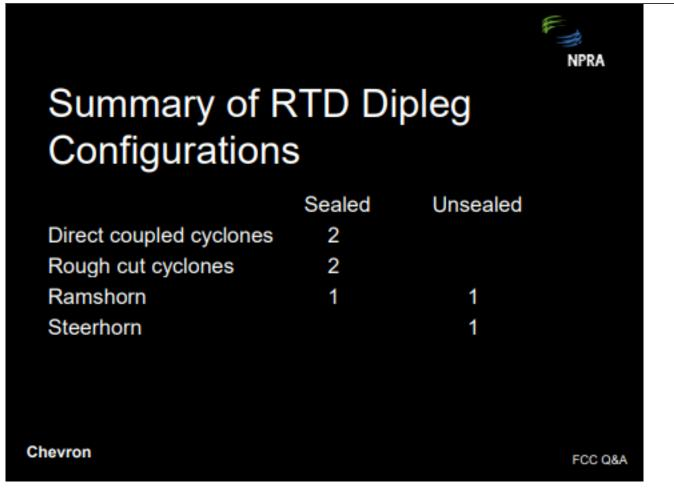
The choice between sealed and unsealed operations is often dictated by the hardware design, since some units can only operate in one mode or the other. For those that can operate either way, the choice is usually dictated by either dry gas make or catalyst losses. We have one unit that starts up unsealed and then switches to the sealed mode when the operation stabilizes.
