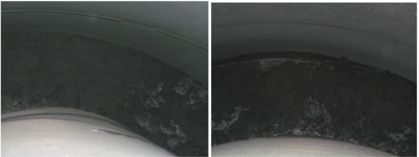
Picture-1: Huge quantity of coke in annular space between reactor grid and shell
