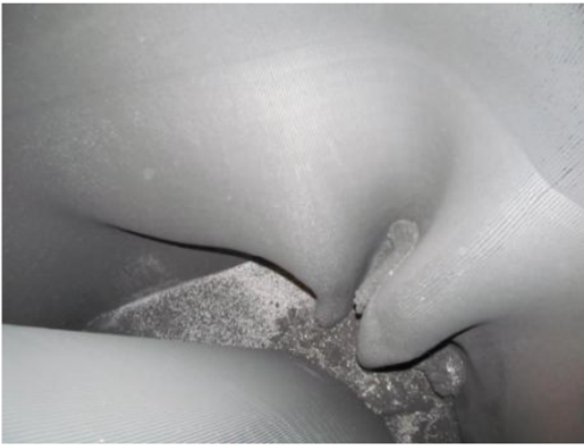
Picture-2(a): Last panel of outside reactor grid found fully bulged with huge coke build up
