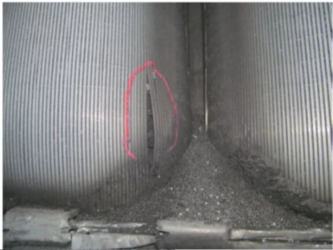
Picture-3(b): Shiny coke between and inside scallops leading to bulging and fish mouth cracks A joint root cause analysis with Licensor confirmed presence of Fe and carbon graphite (high carbon content) in the coke samples. During cleaning of the scallops, presence of lot of hard shining coke (metallic coke) was observed along with soft coke. It was concluded that coke build up in reactors/scallops/grids may have taken place due to metal catalyzed coking considering problem with DMDS dosing pump during initial year of commissioning as well as due to other reliability issues like frequent trip of recycle gas compressor. The presence of metallic coke in reactors may have acted as nuclei and further catalyzed the coke growth during recycle gas failure.
